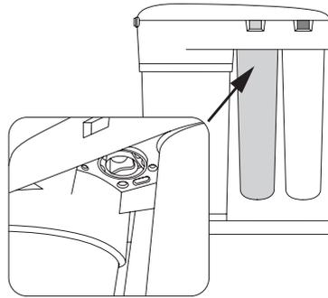
7. Open the clean water faucet and flush the preliminary water treatment cartridges for around 20–30 minutes.
