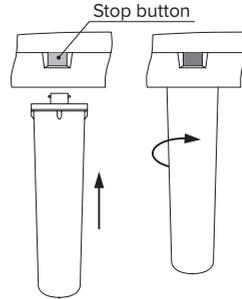
Figure 13. Installation of the membrane cartridge service plug
